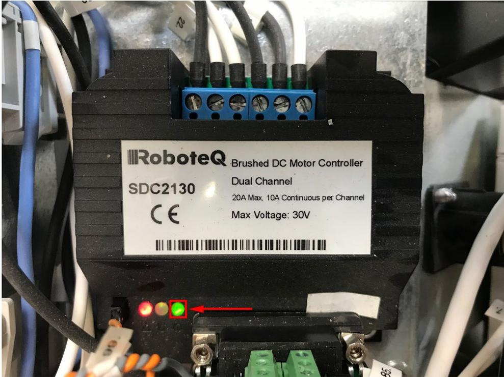
Figure 1.4. Motor controller LED
